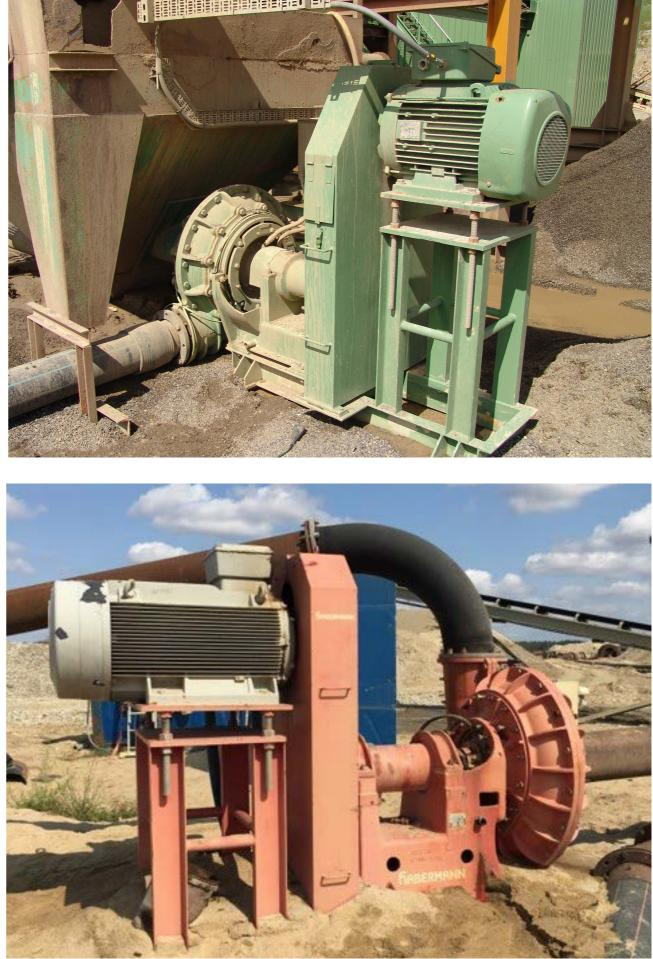
All wearing parts that come into contact with the medium are made of elastic, non-metallic materials and are individually selected according to the requirements in terms of material quality.
