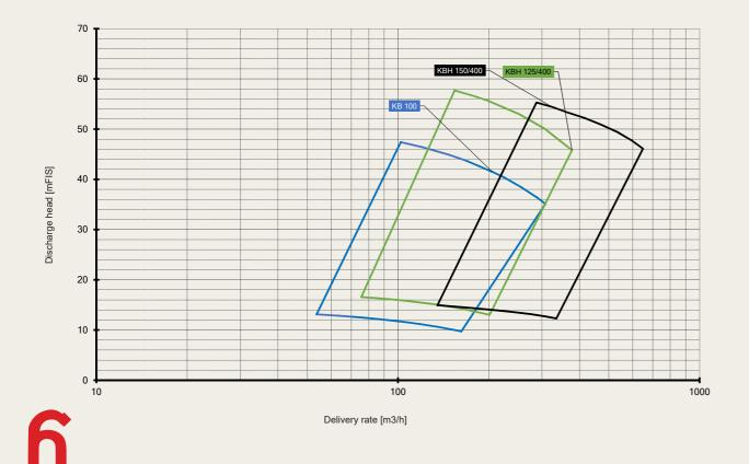
The combination can be adapted to the customer's requirements. The **tunnel version** is used for micro tunnelling in the majority of cases due to the limited space available. The **shaft version** is used as a feed pump or booster pump in the shaft, from the shaft to the separation plant. Shaft versions are more frequently used for larger pipe jacking dimensions, whereby the discharge nozzle settings can be variably adjusted within the technically possible framework.
